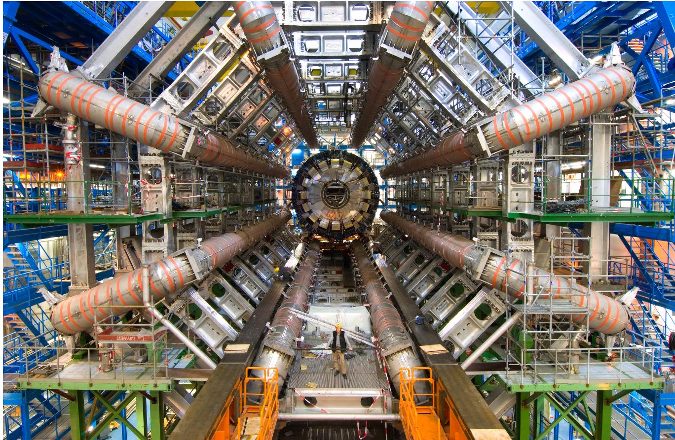
The outer toroidal magnetic field is produced by eight very large air-core superconducting barrel loops and two end-caps. 26 m long and 20 m in diameter, and it stores 1.6 gigajoules of energy. Its magnetic field is not uniform.
