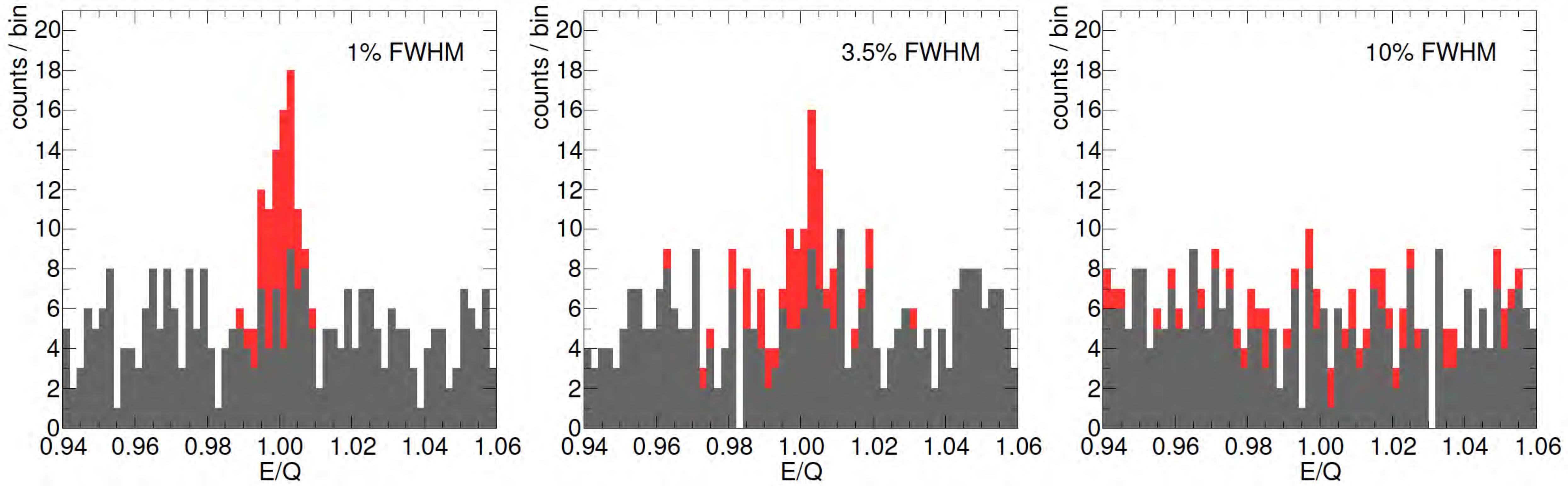
Signal and background (red and grey stacked histograms, respectively) in the region of interest around  $Q_{\beta\beta}$  for 3 Monte Carlo experiments with the same signal strength (50 counts) and background rate ( $1 \text{ count keV}^{-1}$ ), but different energy resolutions: top: 1% FWHM, centre: 3.5% FWHM, bottom: 10% FWHM. The signal is distributed normally around  $Q_{\beta\beta}$ , while the background is assumed flat.
