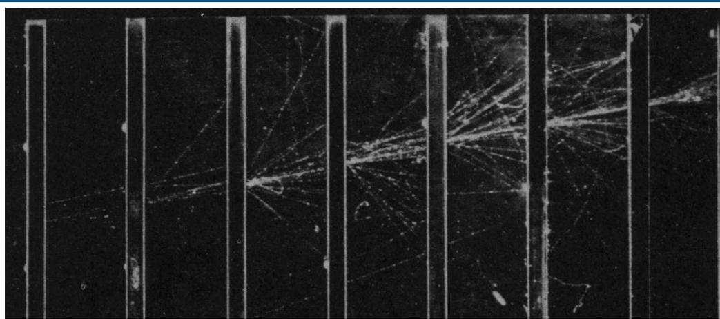
Photon-induced **shower** in a cloud chamber; the intermediate black parts are lead blocks; in addition, there is a magnetic field perpendicular to the figure plane
