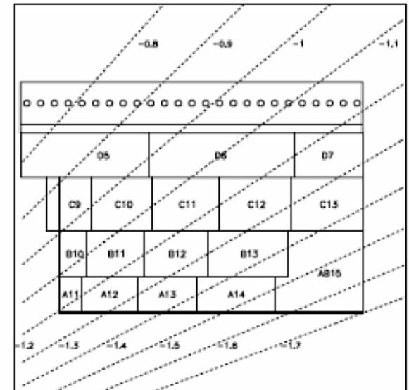
Figure 5-16 Proposed cell geometry for the extended barrel modules (version "a la barrel").
