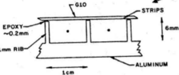
Fig. 3. Prototype strip chamber cross section.
