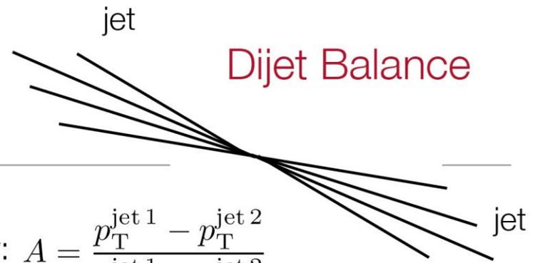
Resolution:  $\frac{\sigma(p_T)}{p_T} = \sqrt{2}\sigma_A$  using  $p_T$  asymmetry:  $A = \frac{p_T^{\text{jet } 1} - p_T^{\text{jet } 2}}{p_T^{\text{jet } 1} + p_T^{\text{jet } 2}}$
