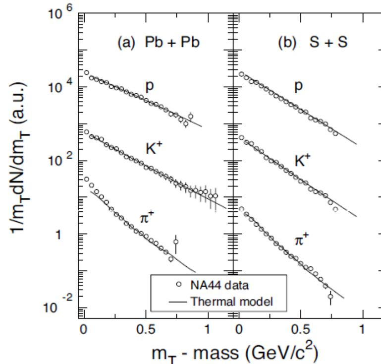
Because of decay products from the resonances, a steeper component exist in low- $m_T$  region for pions. Proton and anti-proton distributions look flatter than those for pions and kaons.
