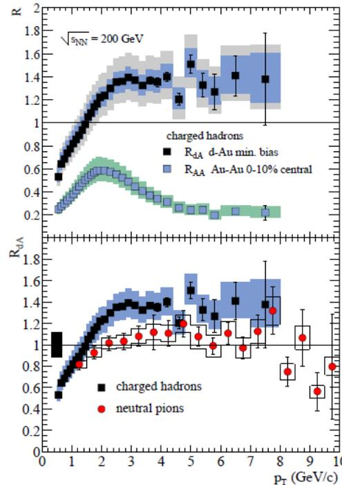
For  $p_T > 2$  GeV one observes a suppression in  $R_{AA}$  consistent with energy loss of partons in the medium
