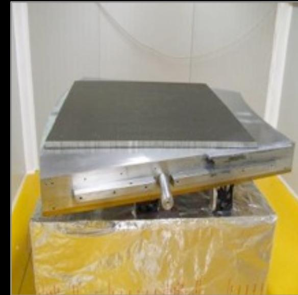
Replica techniques (thin glass sheet on honeycomb structure with aluminized surface), are a cheap possibility, while diamond milled surfaces have a longer life time
