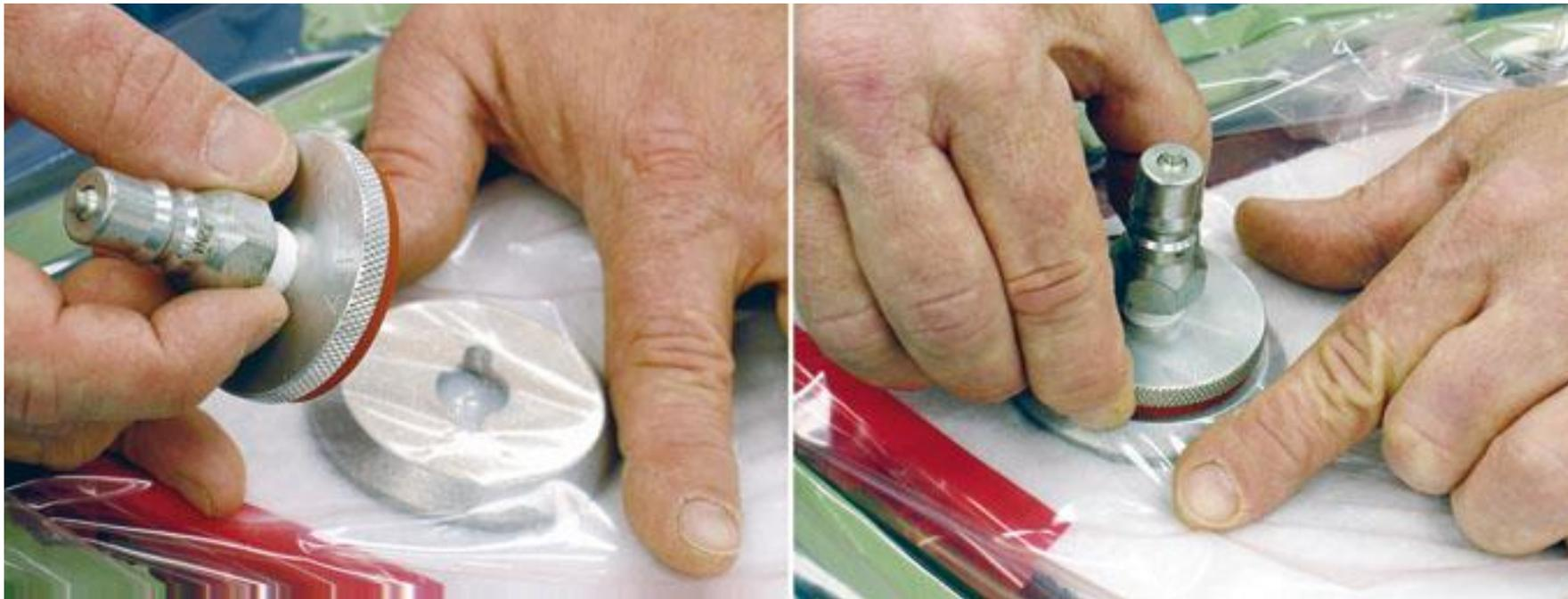
**Foot of vacuum fitting must be inserted into bag:** Remember to do this before completely sealing the bag. Cut a small X where the fitting will penetrate. Find a position on the mold where the fitting will not sit on the part itself. Make sure there is adequate breather for conduction.
