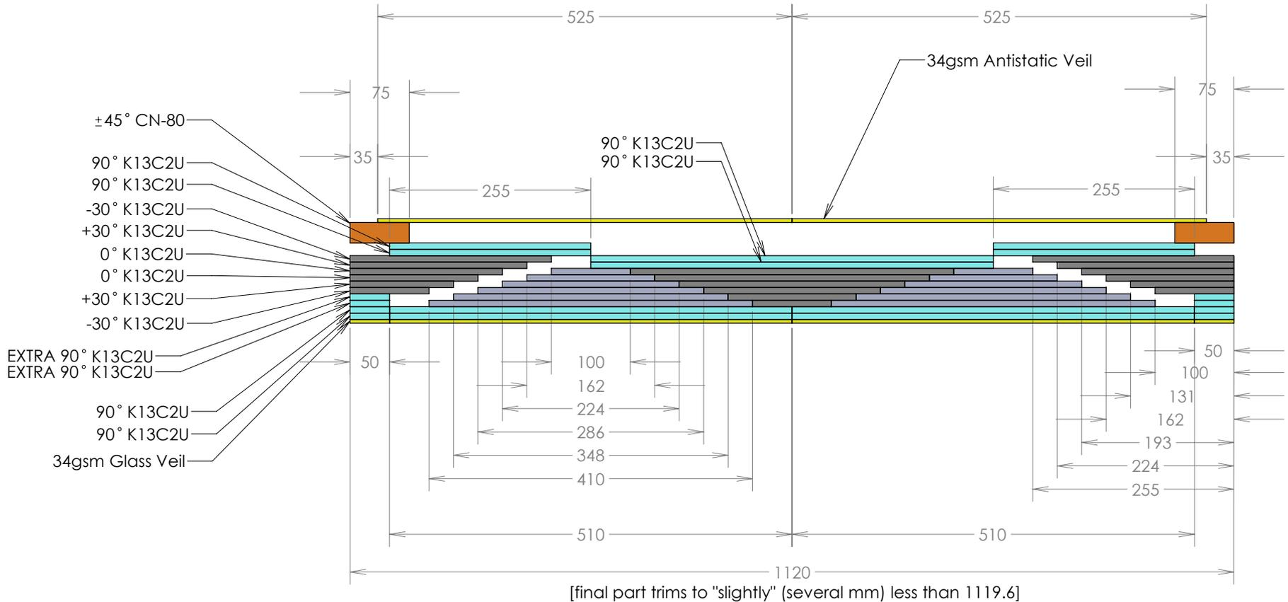
Pre-oriens fibers, makes thin (30-50 $\mu$ m) lamina easier to handle and apply to tool
