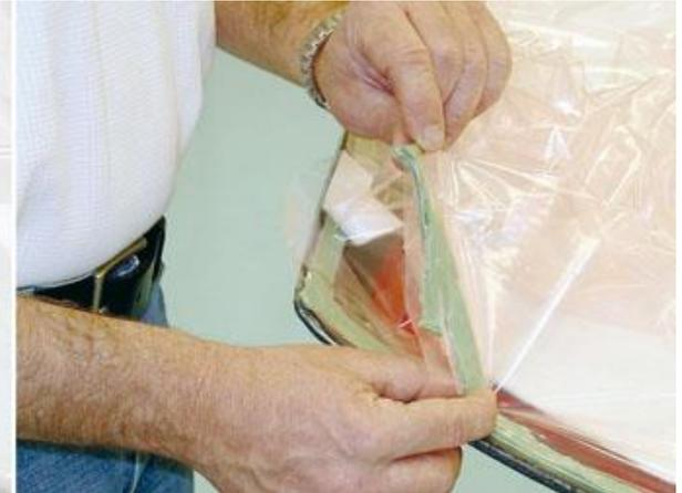
**Sealing Pleats:** Make sure vacuum tape is sealed completely at the root and end of the pleat. These are locations where leaks typically occur. It may help to stretch the pleat while pinching at top and bottom to create the seal.
