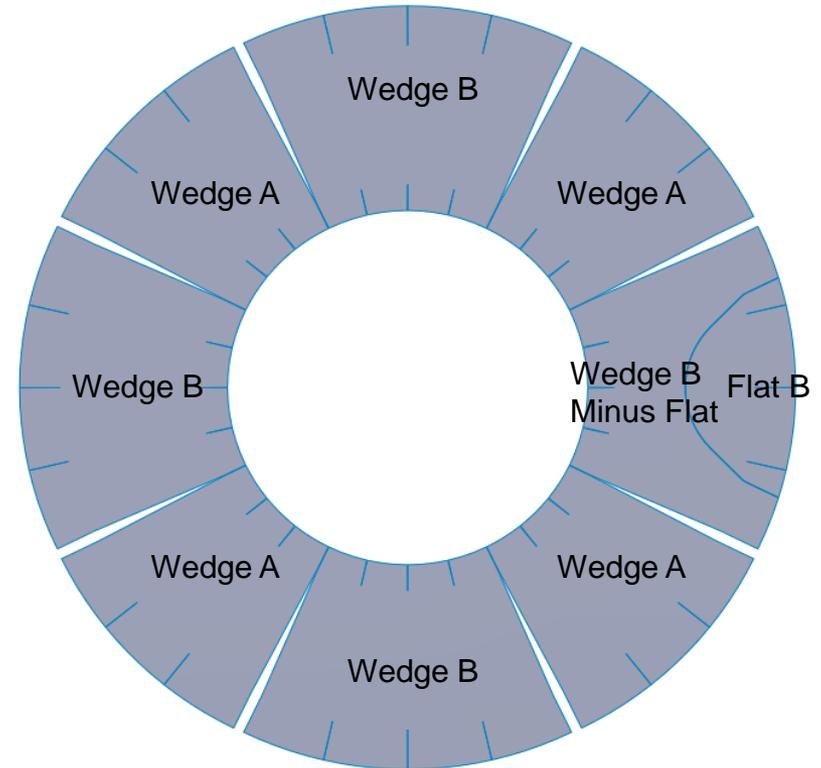
The staggered angle variation ( $38^\circ$  to  $52^\circ$ ) allows good overlap from ply to ply. Half the plies must be cut at  $0/90$ , and half at  $\pm 45$ . 0.5mm gaps are provided between plies.
