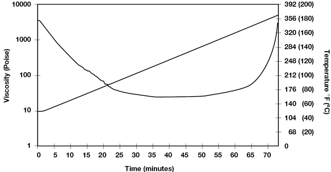
This is a typical viscosity profile— $\mu$  drops first from increased temp then increases from onset of cure and cross-linking—in this case a 350F cure Cyanate Ester system is shown
