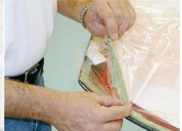
**Sealing Pleats:** Make sure vacuum tape is sealed completely at the root and end of the pleat. These are locations where leaks typically occur. It may help to stretch the pleat while pinching at top and bottom to create the seal.
