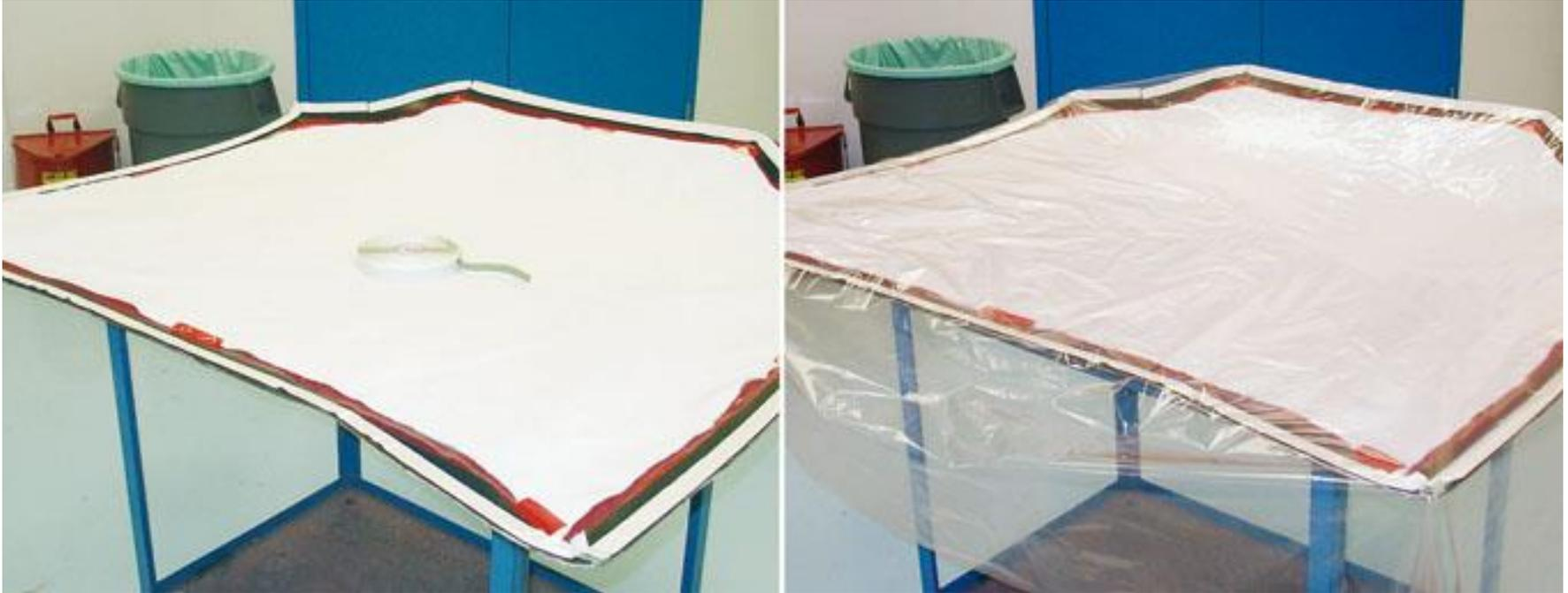
**Bag Sealant (« Tacky ») Tape:** Applied continuously to tool all the way around the part. Must be rolled onto tool for good seal. Can be doubled, but care should be taken to avoid penetrating leaks.
