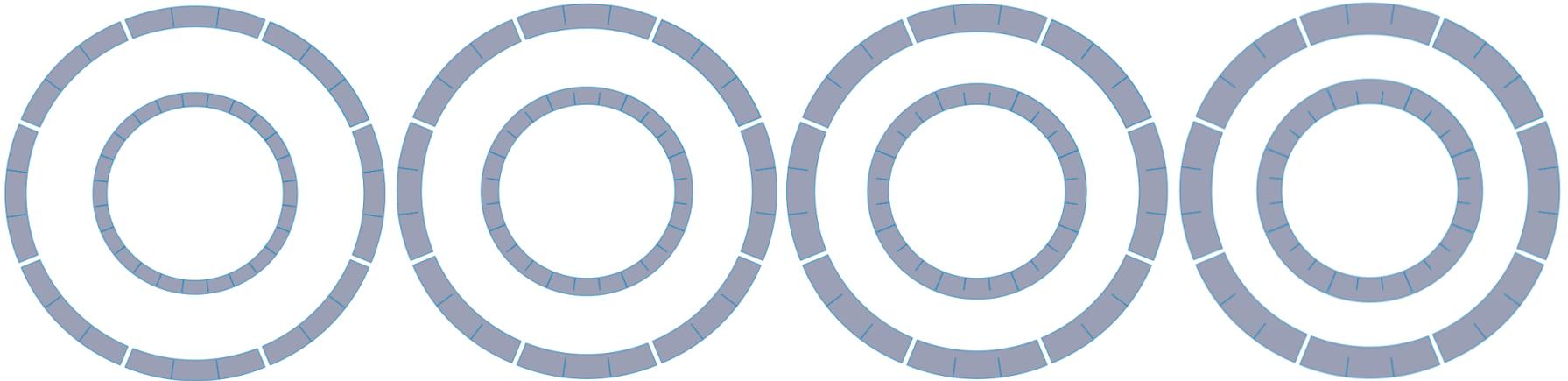
Flanges are thickened by interleaving extra ring plies at the inner and outer radii.
