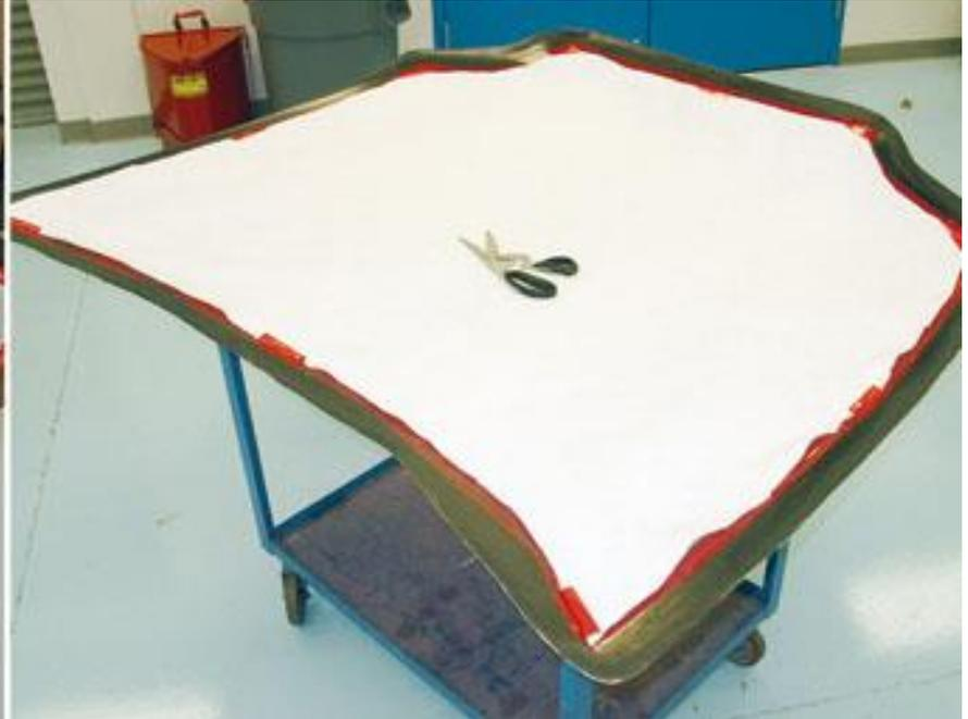
**Release Film (Plastic Sheet):** Can be loosely applied over peel ply, but must not bridge. Can be perforated or not. Prevents breather from becoming saturated with resin, starving laminate, and cutting off vacuum. Perforations allow for greater resin flow/loss. Need to experiment for rich or high-volatile systems.
