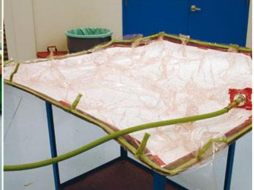
**In a pleat:** Allows placement on any mold, anywhere. However, the pleat must have adequate breather to ensure conduction to the bulk of the tool surface, and it should be strain relieved so as to avoid bridging of the pleat where it contacts the tool.
