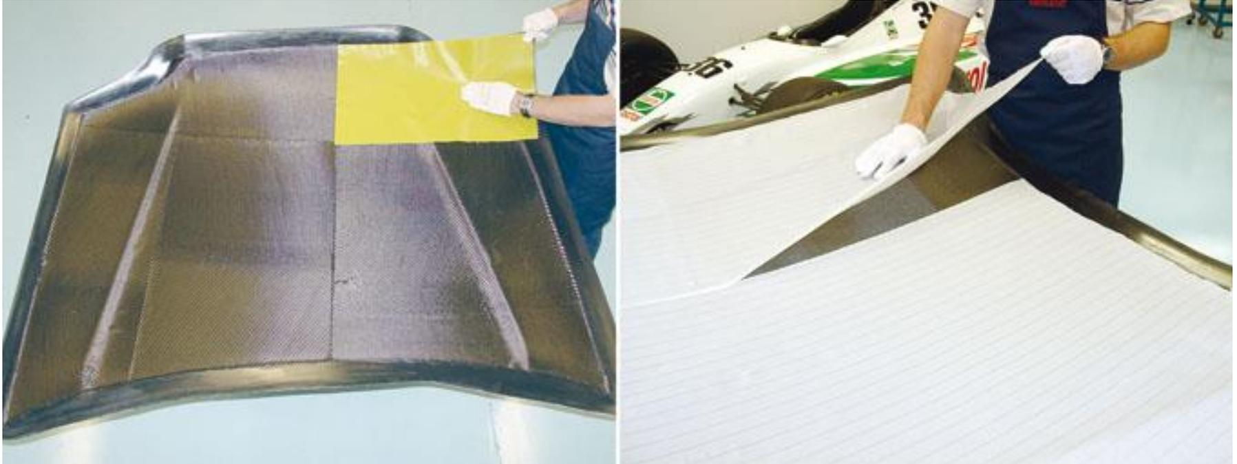
**Peel Ply or Release Ply:** Protects laminate from bagging material, ensures clean release, provides even surface finish. Must be applied *flat* on all surfaces, but *can be joined or overlapped*. This is also the Bleed system to extract appropriate amount of resin.
