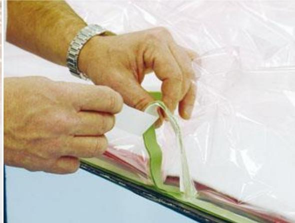
**Creating Pleats:** Pleats will be necessary near corners, curves, and wherever excess bag is bunched up. They are also critical for avoiding bridging on complex shapes. It is preferable to include pleats regularly on the long edges of irregular bag shapes.
