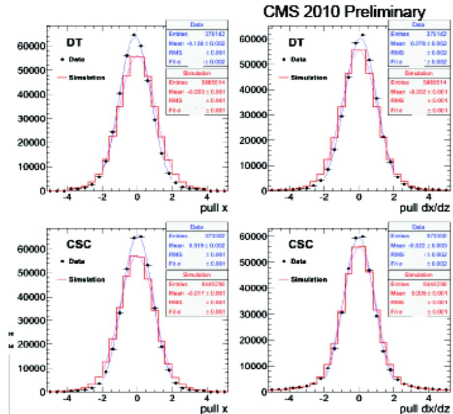
Resolutions of extrapolations from central tracker to muon segments
