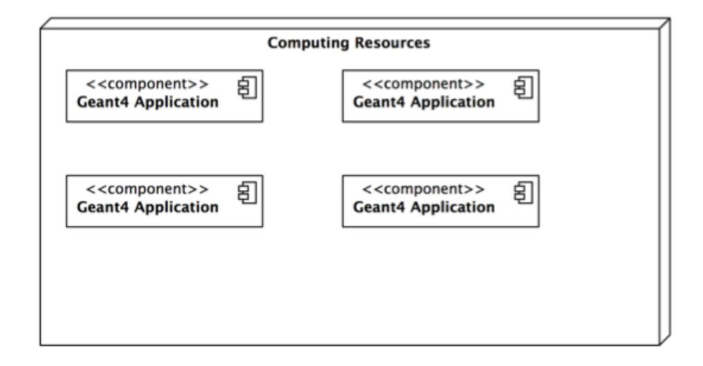
MT Application: single application starts threads. For G4: application (master) controls workers that do simulation, no memory sharing now, each worker is a copy of the application
