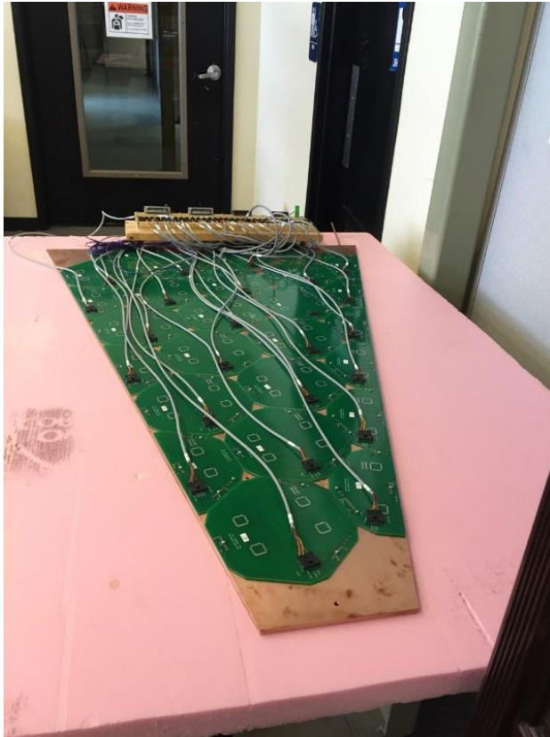
“dummy” cassette for thermal tests
