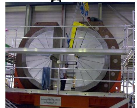
HB/HE: Sampling Brass/plastic scintillator calorimeter
