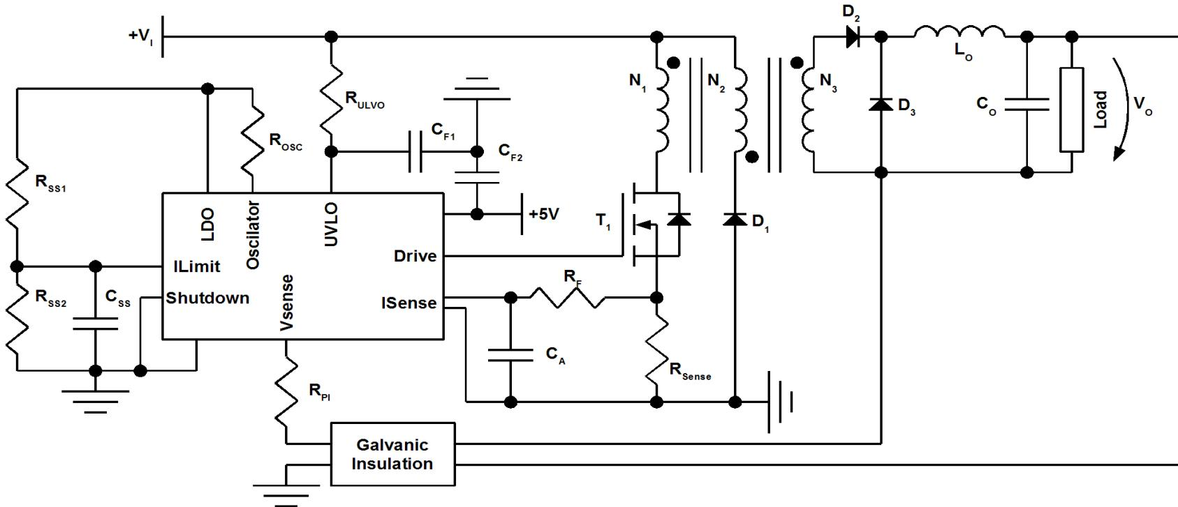
Radiation resistant isolated DC-DC converter using a forward topology
