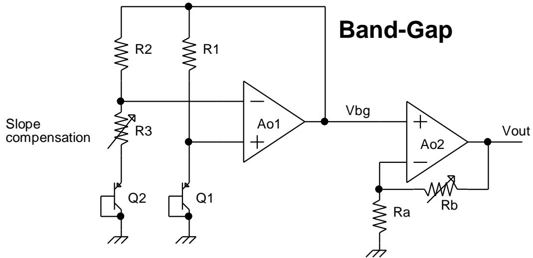
$$V_{OUT} = V_{be_1} - \left(1 + \frac{R_2}{R_3}\right)V_{OS} + \frac{R_2}{R_3}V_T \ln\left(n\left(1 - \frac{V_{OS}}{I_{R2}R_2}\right)\right)$$
