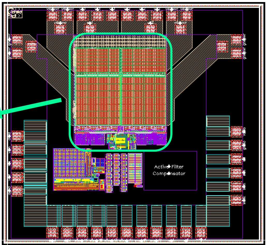
Note: MPW area constrains TC to single channel (1 reticule, 1.52x1.52 mm<sup>2</sup>)
