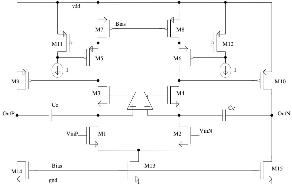
$$V_{namp} = \sqrt{\frac{2}{3}} \frac{K \cdot T}{C_c} \cdot \frac{1 + \frac{V_{dsat1}}{V_{dsat7}}}{f}$$
