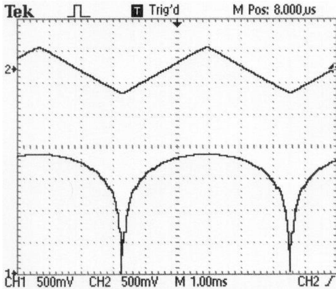
**Measured output of the pipeline converter by injecting a triangular waveform of 250 Hz at the input, for a clock frequency of 1.3 MHz**
