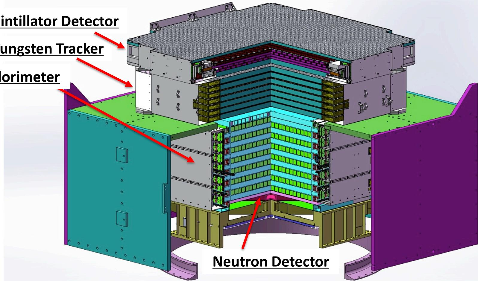
**W converter + thick calorimeter (total  $33 X_0$ )
