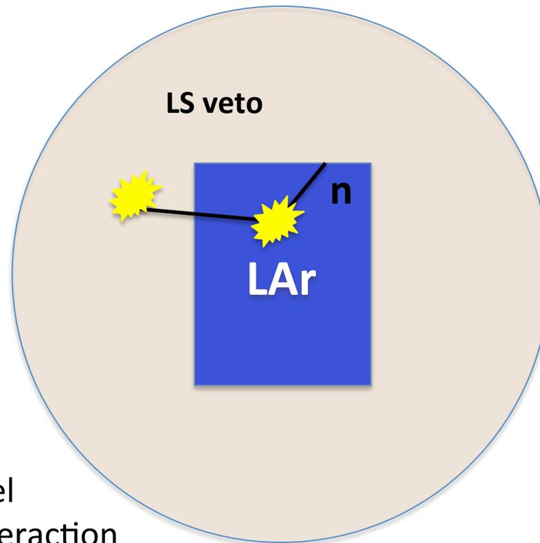
A radiogenic neutron from the cryostat steel or PMTs makes an interaction in LAr (WIMP-like) and later is captured in the LS veto. This type of event is rejected.
