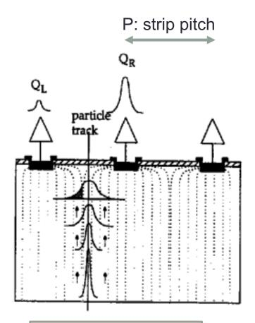
Use the laser system to see how charge is shared between strips. Can
