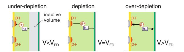
$C = \epsilon \frac{A}{W}$  Noise in the readout electronics grows with capacitance at the input
