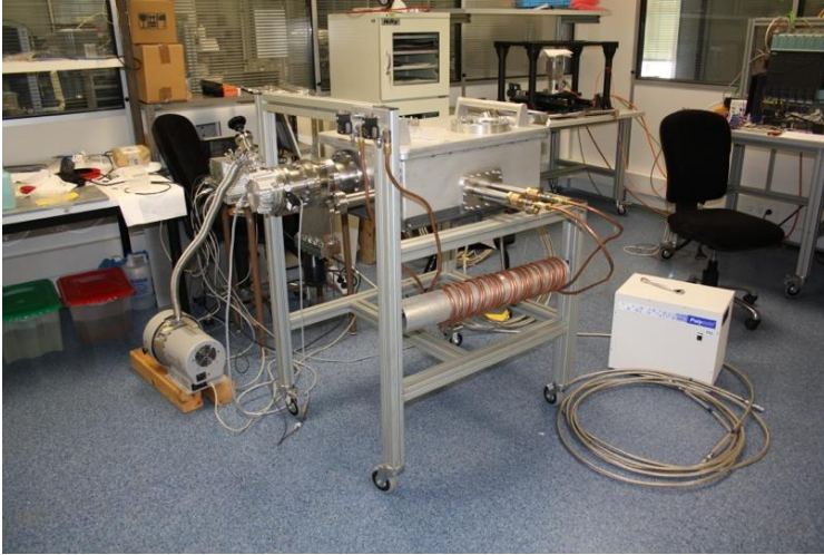
Cryogenics and vacuum tests on prototype
