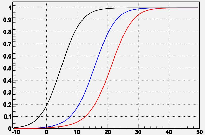
*Real data (now a days irrelevant and forgotten) on scaled transmittance of aerogel tiles under different pressure and temperature*
