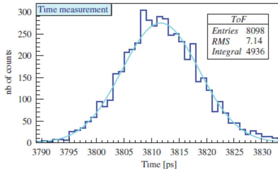
Fig. 13. Time-of-flight measurement at GSI with an  $^{238}\text{U}$  beam at 600 A.MeV. Start detector:  $150 \times 32 \times 1 \text{ mm}^3$ , Stop detector:  $600 \times 32 \times 4 \text{ mm}^3$ . Only H6533 PMTs are used for that measurement.
