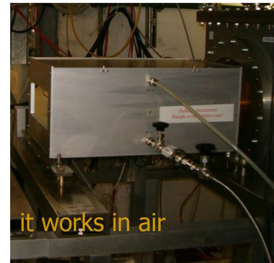
Three sets of preamplifiers are supplied to cover the complete dynamic range of the charge signal from  $Z=92$  to  $Z=3$  (variation by a factor  $10^3$ ).
