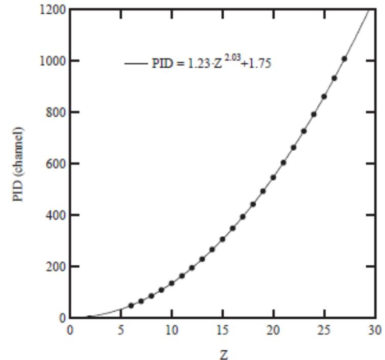
Fig. 4. PID vs. Z relationship for  $A/Z = 2$  nuclides. A solid curve is the best fit to the PID and indicates that the PID is proportional to  $Z^{2.03}$ . The errors of the PID channels are less than the marker size.
