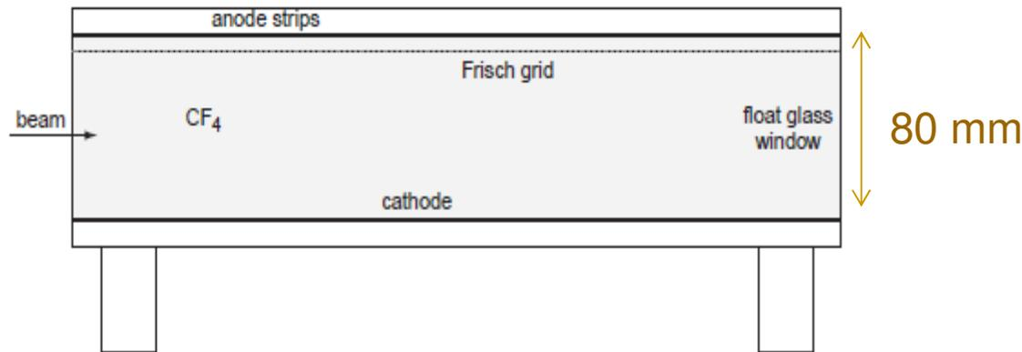
Tested successfully for particle rates of up to 200 kHz, thanks to a 10th order shaper which returns very fast to zero line and an overall DC-coupling is used, which avoids rate dependent baseline drift.
