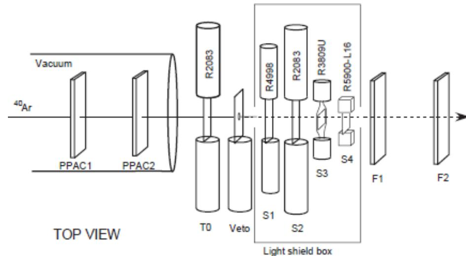
Optimization of scintillation detector for heavy ion beams indicates higher timing resolution scaling by the pulse height and the number of photoelectrons  $N$  produced at the photocathode ( $\sigma_t \propto 1 / \sqrt{N}$ ).
