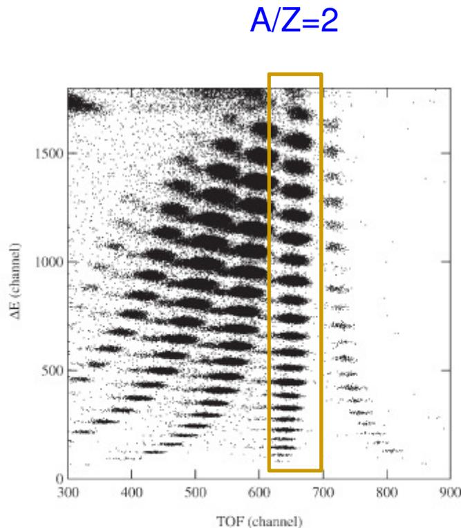
Fig. 2. Two-dimensional scatter plot of  $\Delta E$  vs. TOF for the secondary beam produced by nuclear fragmentation of  $^{56}\text{Fe}$  at 90 A MeV.
