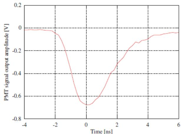
Fig. 6. Example of a PMT output signal waveform.
