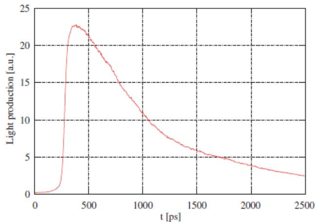
Fig. 5. Typical response from the streak camera. Measured rise-time=40 ps, decay-time=550 ps.
