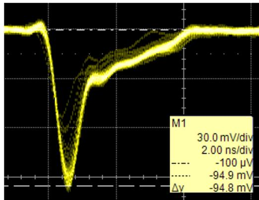
Analog signals, Au beam, HV: 100V
