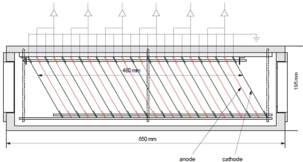
Electrodes plates **tilted** (30°) in order to avoid recombination
