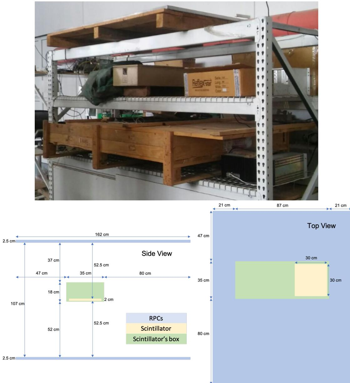
**Figure 9.3:** Top: Hodoscope prototype stand in the Observatory’s assembly building. The RPCs are placed on the higher and lower shelf, separated by 1.07 m. On the middle shelf, inside a wooden box is the small scintillator. Bottom: Representation of the side (left) and top (right) views of the prototype hodoscope setup. The scintillator used to assess the system’s performance is also shown.
