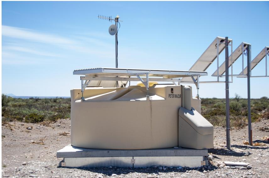
**Figure 4.7:** Peter Mazur SD station in the Infill with MARTA RPCs installed inside the support concrete structure. Extra solar panels and batteries were mounted to not interfere with the standard operation of this WCD.
